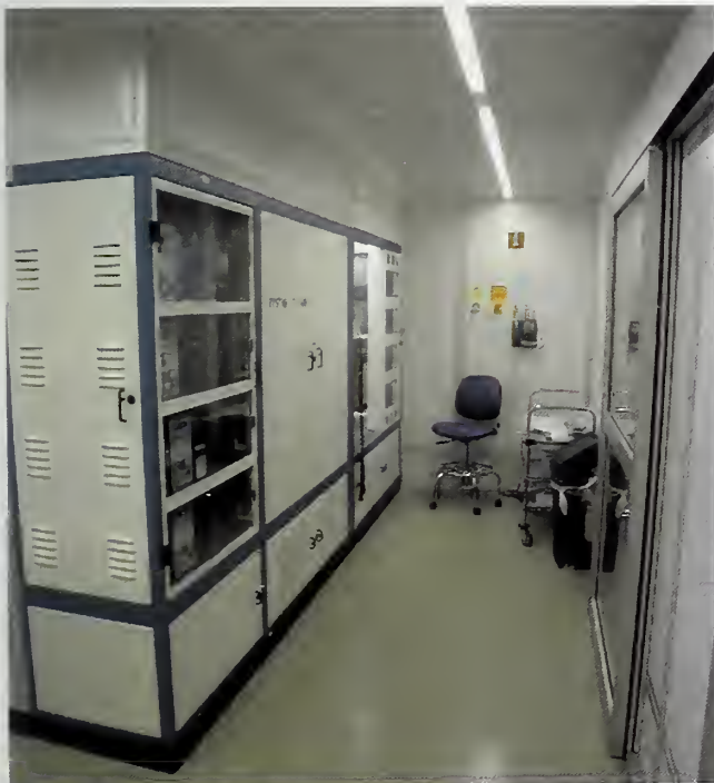
Figure 3. Access bay for diffusion furnaces used to fabrication many MEMS structures for integrated structures that make state-of-the-art standards and measurement technologies possible.
